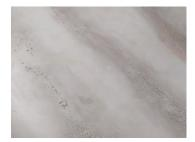
Apply  $2^{nd}$  coat by stainless steel trowel homogeneously on the whole surface in a thick layer (consumption  $1.4 - 1.7 \text{ kg/m}^2$ ), let it dry for 10-20 minutes depending on temperature and humidity, then create the pitted design with Doormat tool. Wait 20-40 minutes before polishing the surface by stainless steel trowel. Polish the surface with flat blade, not with the side of the blade as you would normally do with lime plaster.
